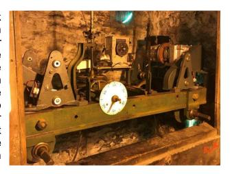
As detailed in Brian's clockmakers report, the tower is suffering from worsening damp caused by unglazed holes in the stonework letting in the weather. As you can see from the photographs below, the water ingress has already started to have a detrimental affect on the clock and timber beams which support parts of the peripheral clock system. The tower as a whole should be assessed by qualified professionals, made waterproof, and any rotten timbers replaced.
